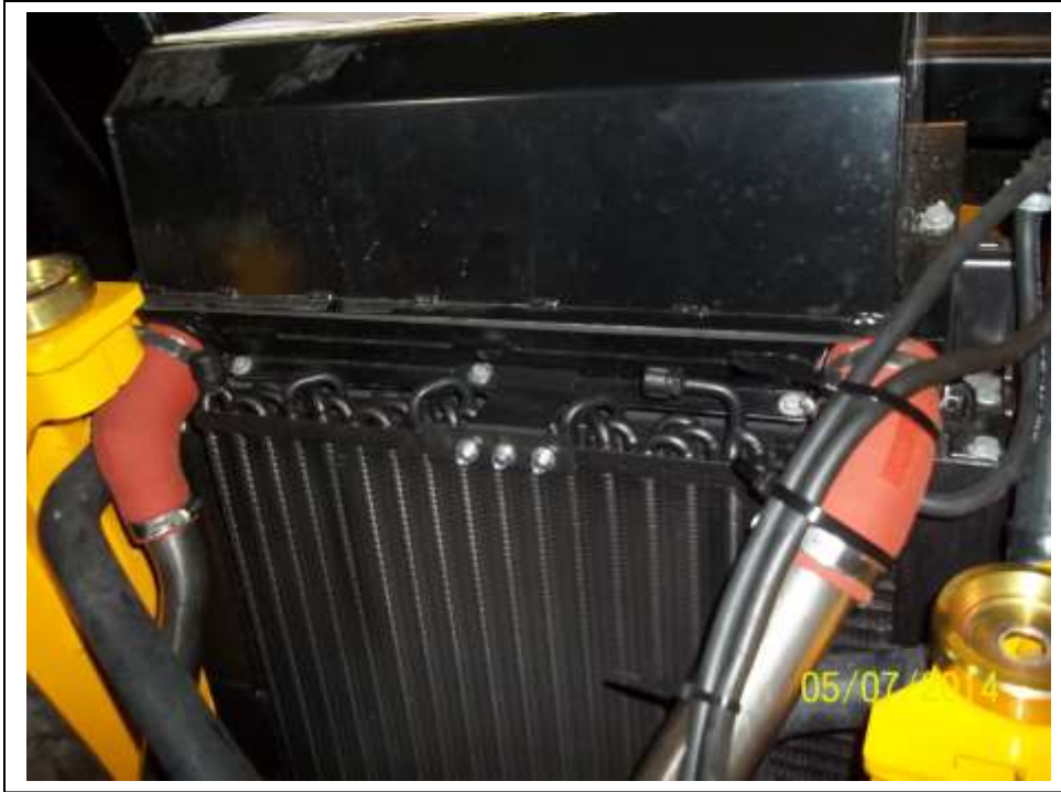
Condenser bolted at top end as shown with one center bracket at the top.
